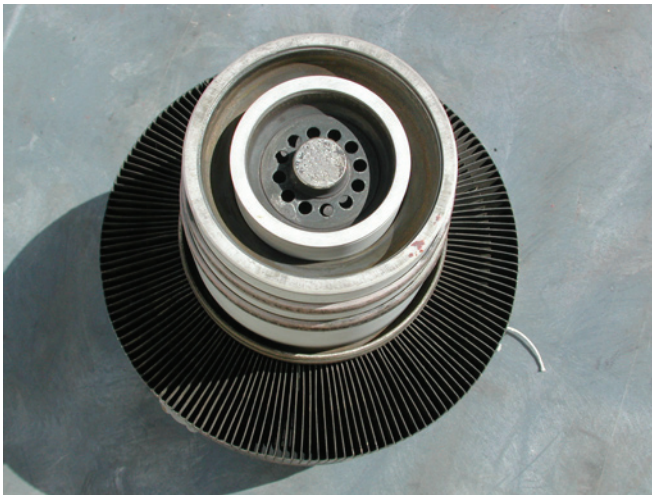
Figure 6 This tube appears to have been in a socket for only a short time, but already has evidence of overheating. Note the discolored stem and anode fins. This tube will have a short lifetime.
