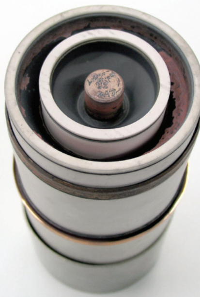
Figure 4 Tube with evidence of overheating. Note the severe discoloration in the tube stem. This tube will have a very short lifetime.
