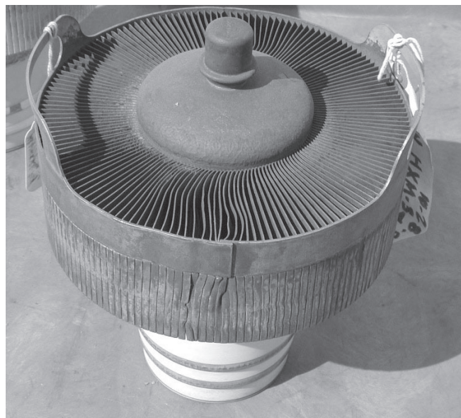
Figure 3 Example of a severely overheated tube. The cooling fins are discolored and badly distorted. This type of overheating will cause premature tube failure.
