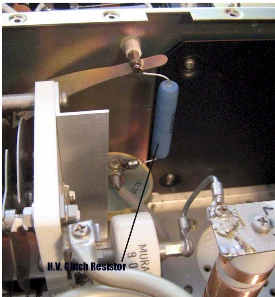
Original inductor L2 replaced with a 10 ohm 'glitch' protection resistor in high voltage supply.
